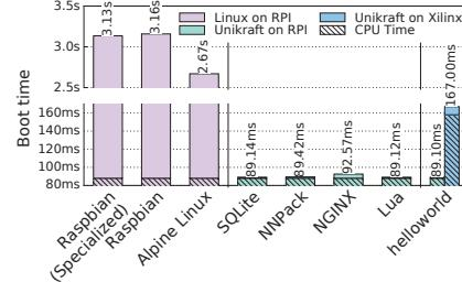
Fig. 4: Boot times of different applications on Unikraft vs. those same applications running on Linux Alpine and Raspbian.
