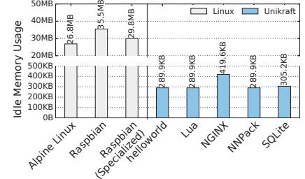
Fig. 5: Idle memory consumption for different applications on Unikraft vs. Alpine and Raspbian.
