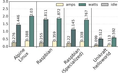
Fig. 3: RPI Unikraft power use vs. Alpine and Raspbian when idle and when calculating  $\pi$ .
